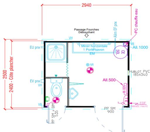
**Dimension: L2940mm x l 2500mm x H 2700mm HSP 2266mm - Panneaux 35mm**
