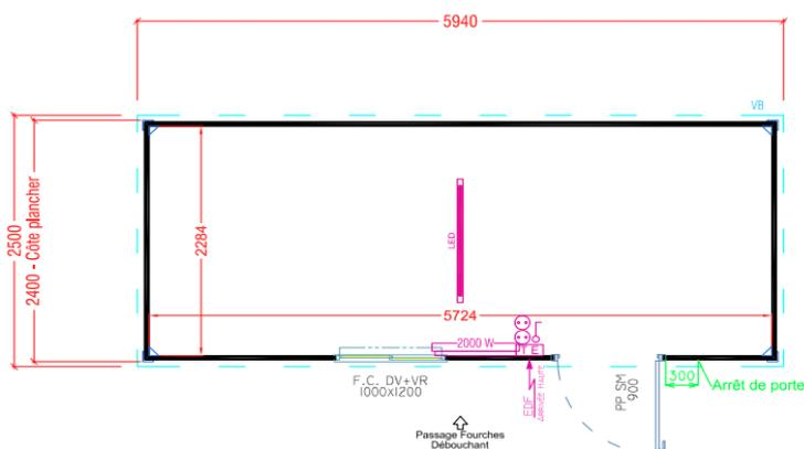
**Dimension: L5940mm x l 2500mm x H 2700mm HSP 2266mm - Panneaux 35mm**
